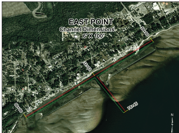
Figure 7-3B. Eastpoint Channel dredge project limits (source: USACE, Mobile District).
