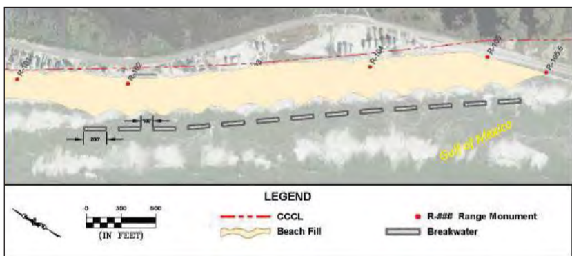
Figure 6-2C. Proposed breakwater alignment plan view (MRD Assoc, 2017).
