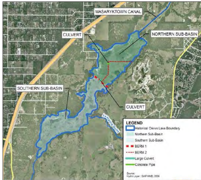
Figure 15-7C. Crews Lake schematic of wetland rehydration engineering plan.
