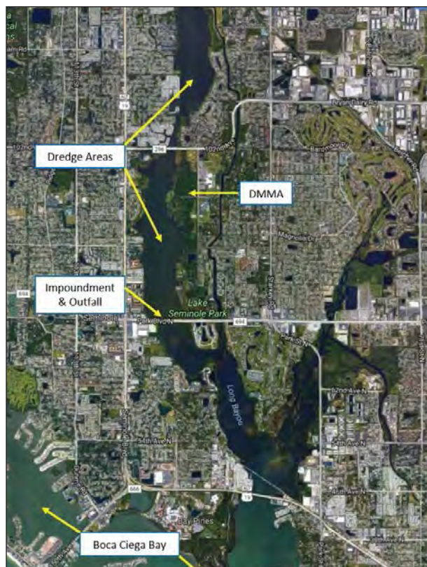
Figure 16-1B. Location of Lake Seminole dredge areas, lake impoundment and outfall, and the DMMA.
